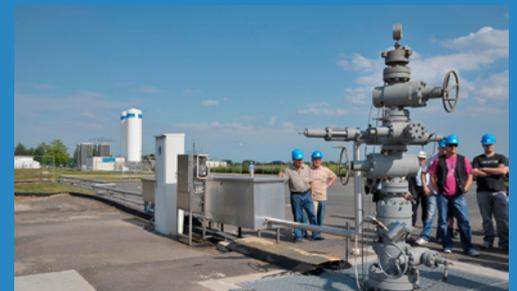
View of the Ketzin pilot injection site, showing the injection well.
